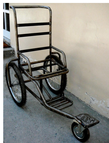
Trike designed by HWI and built in Pakistan. Local materials and manufacturing were used.
